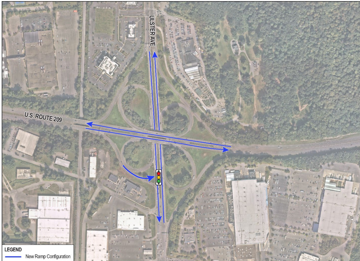
FIGURE 3.3: SIGNALIZED EASTBOUND RAMP CONCEPT
