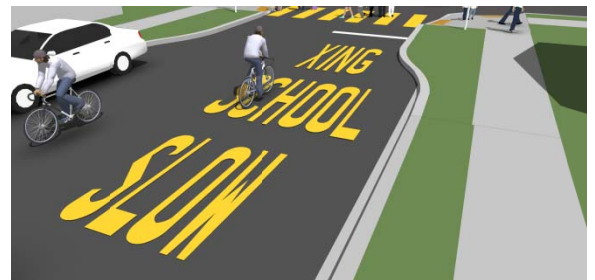
Advanced School Crossing Pavement
