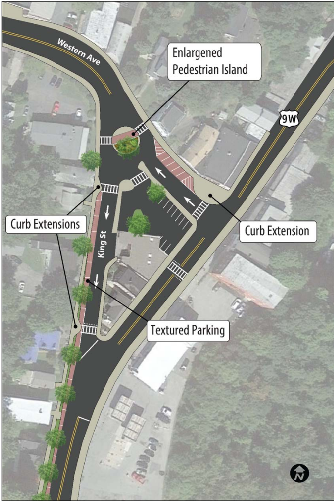
Figure 16: King Street Triangle Alternative 1 – Mini Traffic Circle Concept Source: Alta Planning + Design
