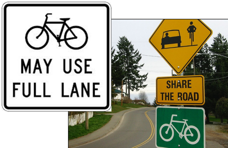
Images 17 & 18: Left MUTCD Sign R4-11 “Bikes May Use Full lane” Source: MUTCD
