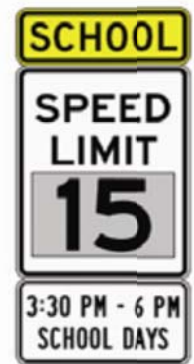
Figure 2: A New York State MUTCD approved school speed limit sign, figure number 7B 100. Source: NYSDOT
