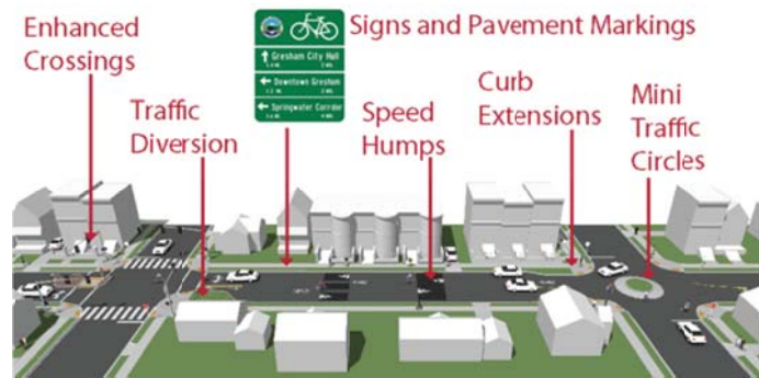
Figure 21: Range of possible treatments to create a Bicycle Boulevards - Source: Alta Planning + Design
