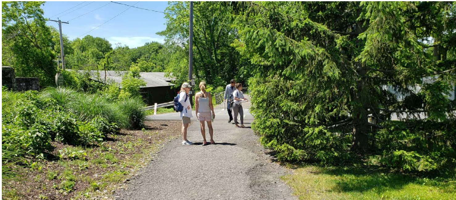
Existing evergreen tree prevents trail users heading south to see approaching vehicles traversing west at Water Street.
