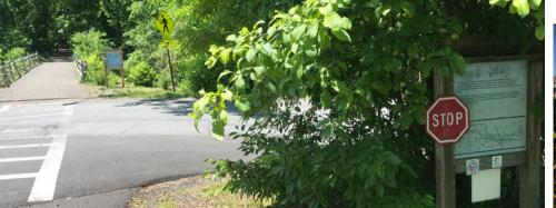
Approaching Water Street from the south, there is a trail sign with a "Caution Road Crossing" sign attached. Given the converging of three vehicular roads with limited sight distance intersecting with a busy pedestrian/cyclist crossing, a stop sign for the trail and vehicular control signs should be considered to prevent conflicts between vehicles and trail users.
