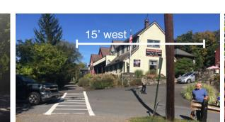
Approaching Water Street from the south, the sight line to the west barely meets the minimum distance required. Given the limited visibility of the vehicles approaching the WVRT from this direction, increased visibility by re-locating the sign and pruning vegetation should be considered.
