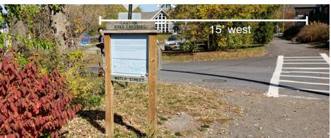
Approaching Water Street from the south, the sight line to the east exceeds the minimum distance required. However, given the limited visibility of the vehicles approaching the WVRT up a hill from this direction, improved signage should be considered.
