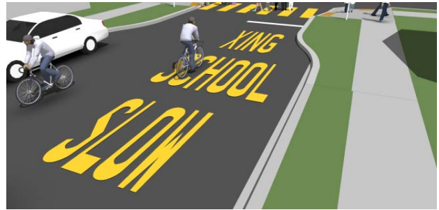
Advanced School Crossing Pavement Marking
