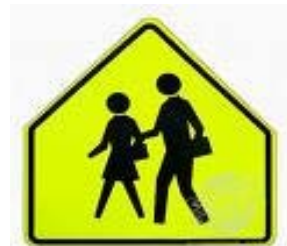
School advance warning assembly from the MUTCD figure S1-1.
