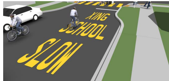
Advanced School Crossing Pavement Marking
