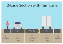
Lane reconfiguration from 4-Lane Section to 2-Lane Section with Turning
