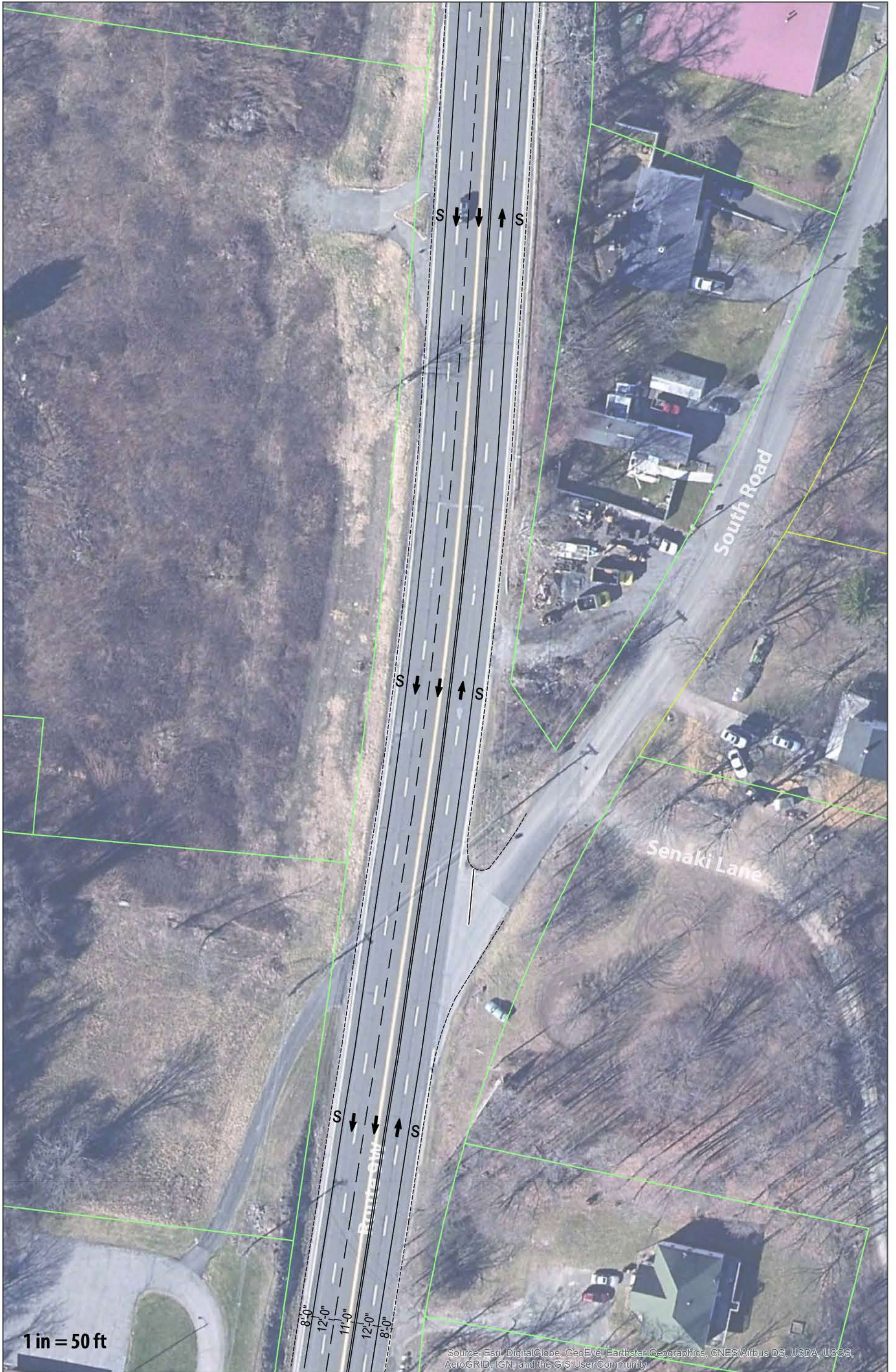
Map 9: South Road (S) Proposed Lane Reconfiguration for Route 9W
